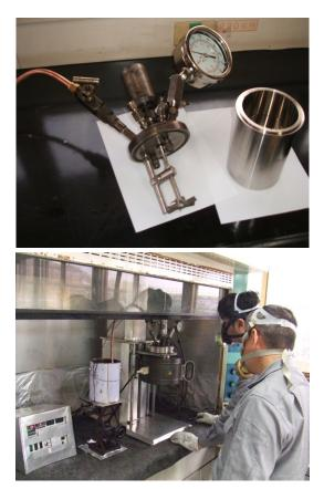
**Fig.2.** Photographs of the Parr vessel and the exper-imental system.
