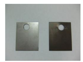
**Fig.10.** The carbon steel specimens: original (left), and, with a full protective film (right).
