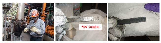
Fig.12. Photographs of the anti-corrosion film formed on the surface of a coupon.
